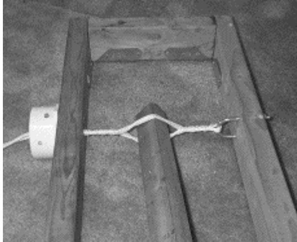
Fig. 5. The open twisted bundle configuration when cocked.
